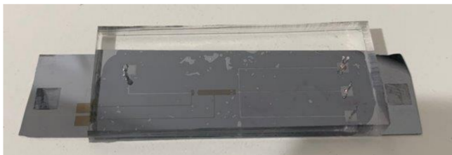
Fig. 2. Final fabricated flow cytometer wafers.
